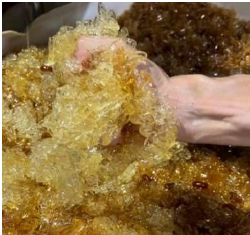
Photo 3: Picture of fish oil pills after running through screw press with no free oil left.
